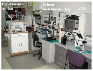
instrumentation for DC (Princeton Applied Research) and AC electrochemistry (Solartron). In addition, Professor Pesic may acquire his own benchtop SEM/TEM microscope (LVEM5). The major advantage of having own equipment is that the students do not have to sign up and have long waiting periods to do their research, as typically found in centralized user facilities.
