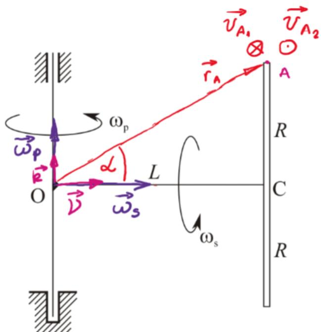
$$\vec{v}_A = \vec{\omega} \times \vec{r}_A = \underbrace{\vec{\omega}_p \times \vec{r}_A}_{\vec{v}_{A1}} + \underbrace{\vec{\omega}_s \times \vec{r}_A}_{\vec{v}_{A2}}$$
