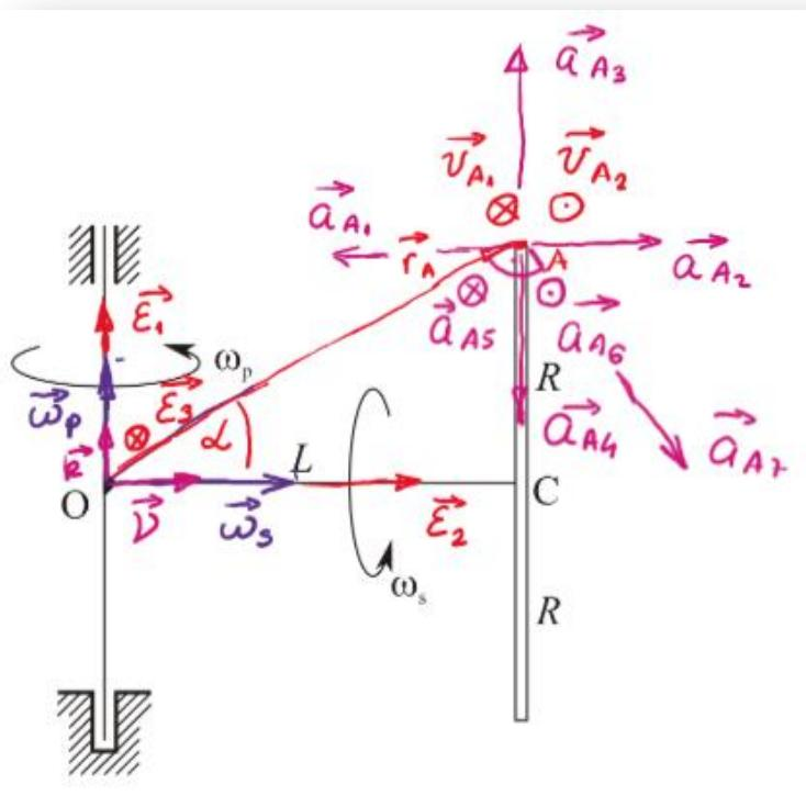
$$\vec{a}_A = \underbrace{\vec{\omega} \times \vec{v}_A}_{\vec{a}_\omega} + \underbrace{\vec{\epsilon} \times \vec{r}_A}_{\vec{a}_\epsilon}$$
