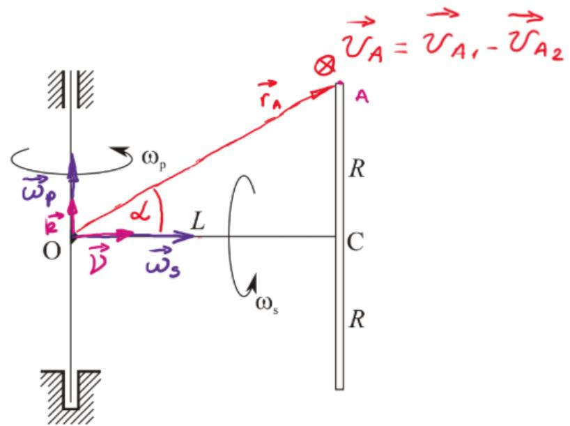
$$v_A = v_{A1} - v_{A2} = L\omega_p - R\omega_s$$
