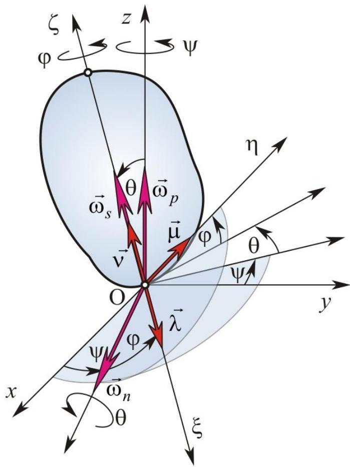
$$\vec{\omega} = \omega_p \vec{k} + \omega_n \vec{n} + \omega_s \vec{v} = \dot{\psi} \vec{k} + \dot{\theta} \vec{n} + \dot{\phi} \vec{v}$$
