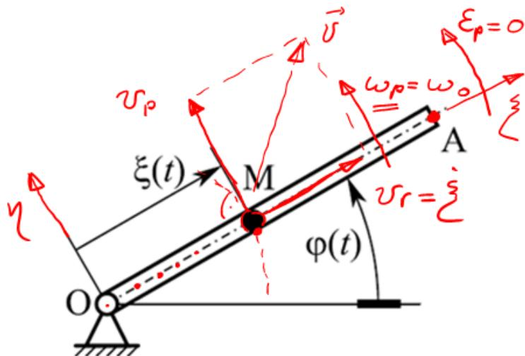
$$\begin{aligned}\varphi(t) &= \omega_0 t \\ \xi(t) &= \frac{L}{T} t \\ \vec{v}_H(T) &= \vec{v}(T) = ? \\ \vec{a}_H(T) &= \vec{a}(T) = ?\end{aligned}$$
